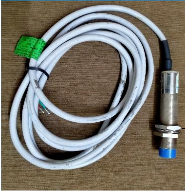
Tech. Specs- NO Type; 8 to 24 v; 3 wire
