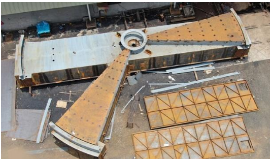
TYPE O– JOB - Tri-Sector Plate Assembly Industry – Power Plant HEIGHT AND Width – 2.5 M Height and 16 Meter length, 4 meter width in dismantled condition W–IGHT - 241 approx. approx
