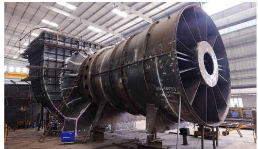
TYPE O– JOB - FGD Fans Statics Industry – Power Plant HEIGHT AND Width –9.5 Meter and width 7 242pprox.approx. & length 20 242pprox.approx. in assembled condition W–IGHT - 242pprox.approx. in assembled condition
