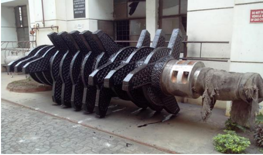
TYPE OF JOB - Sinter Breaker Shaft Industry – Steel Plant HEIGHT AND WIDTH – 2 Meter Height and 2 Meter by 12 Meter width WEIGHT – 40 MT approx.
