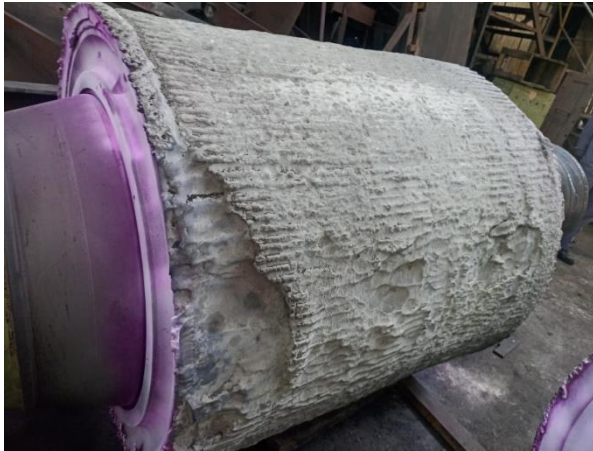
Roller Press Roll - Worn out
