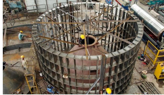
TYPE OF JOB - Separator Rotor Industry – Cement Plant HEIGHT AND Width –4.5 Meter and 6 Meter Diameter WEIGHT - 15 MT approx
